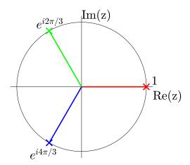
We now define the root-finding problem to be f(z) = 0, where  $f(z) = z^3 - 1$ , with derivative  $f'(z) = 3z^2$ . Newton's method for determining the three complex roots of unity is given by the iteration
